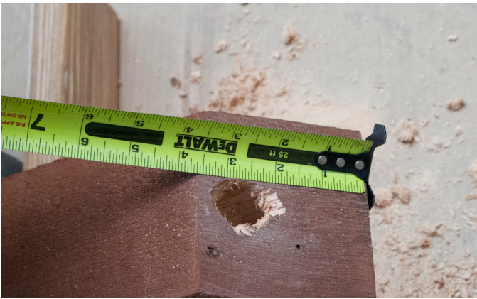
Measure from the bottom point of the Diagonal Web to the center of the hole.
